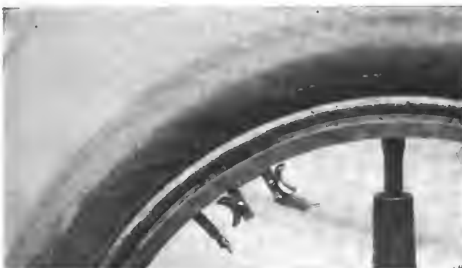
CLIP WHICH HOLDS ENDS OF AJAX RIM TOGETHER.
